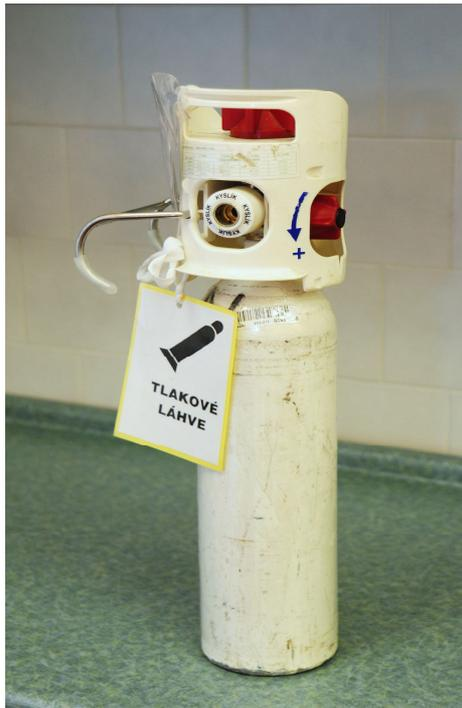
Fig. 16-3: Oxygen cylinder with integrated valve (LIV)
